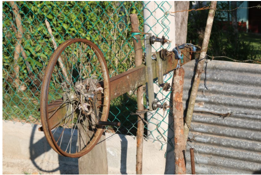
Home made machine for spinning thread into string for hammock weaving.
